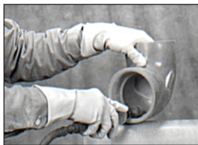
High speed die grinder for sanding sockets. Use drum with 36-60 grit abrasive.
